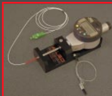
Ferrule measurement system verifies compliance to length specifications
