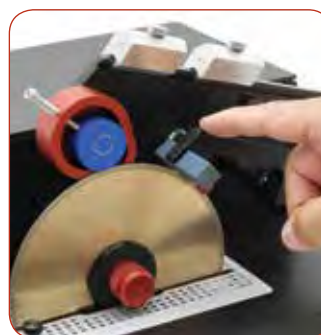
Spring-retractable dressing stick attachment allows dressing while sectioning.
