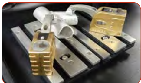
Dual T-slot tables provide a versatile platform for various fixturing options to secure irregular-shaped samples (#5-4050 Vertical Adjusting Clamps shown).
