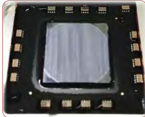
Flat plane deprocessing produces nonuniform material removal and thickness.
