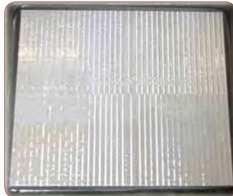
Deprocessing the device by following its profile ensures uniform material removal.
